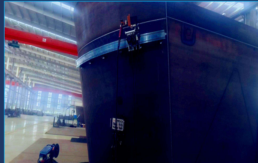
Automated Robot Welding Large Structural Components
